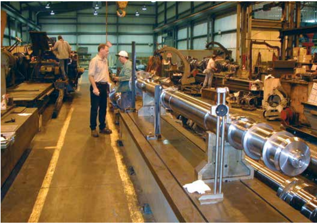
Replacement shaft (14 inches in diameter and 26 feet long) for a Leffel horizontal unit in Indonesia.
