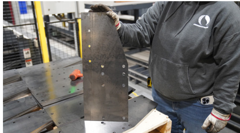
A tower leg component, cut by laser.
