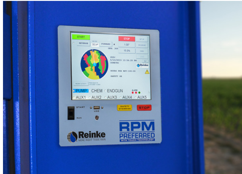
A Reinke touchscreen control panel demonstrating a variable-rate irrigation program.
