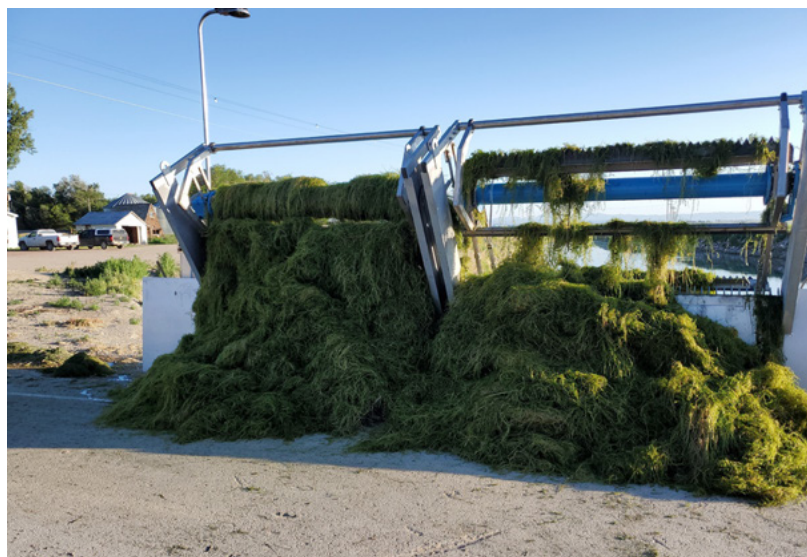
FlexRake Heavy Duty handles the heavy inflow of moss from the lake at Owsley Canal.
