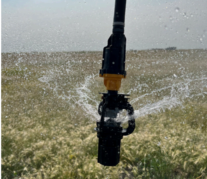
The KPT PC-180° part circle sprinkler in use on a drop in Alberta.
