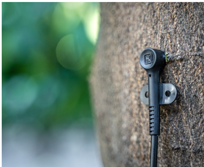
Installing Transpira involves drilling a 4-millimeter pilot hole into the tree, inserting a sensor, and entering basic parameters about the tree into the installation app. It takes less than 10 minutes per site.
