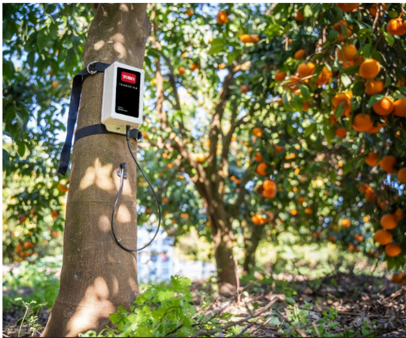
Transpira uses a sensor installed directly in a tree to measure the transpiration process, providing insights into how much water the crop is using.
